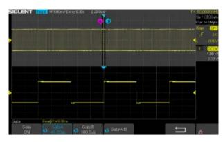
Through Gate and Zoom measurement, you can specify arbitrary waveform interval of data analysis and statistics to avoid measurement errors caused by invalid data.
