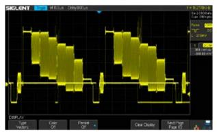
256-level intensity grading display on waveform
