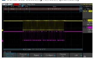
SDS1000X-E displays the decoding through the events list. Bus protocol information can be quickly and intuitively displayed in table form.
